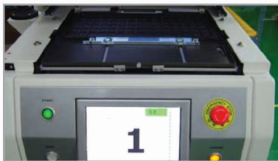
View of a pallet which has moved up to the upper change rack from the STF-100N model after all the materials in it were exhausted
