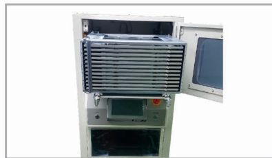
View of the upper magazine of the STF-100D model which is open to refill materials
